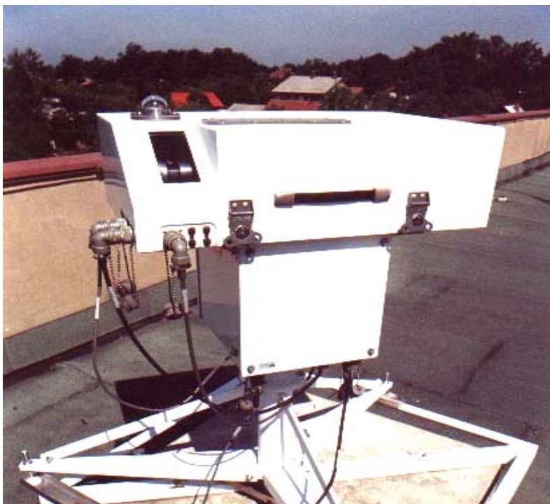
Figure 4. The Brewer MARK-IV spectrophotometer B098 operated at the Solar and Ozone Observatory in Hradec Králové
