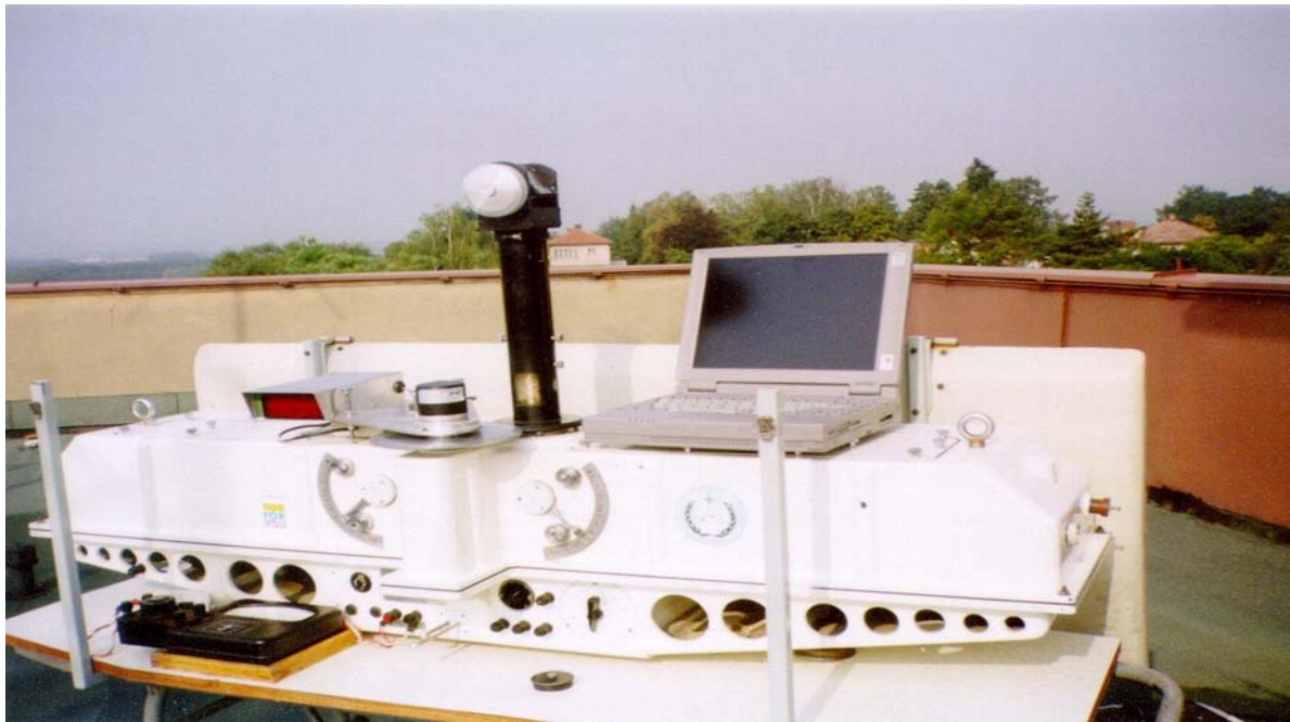
Figure 1. The Dobson ozone spectrophotometer D074 operated at the Solar and Ozone Observatory in Hradec Králové equipped with the semi-automated facility for data recording and processing of observations
